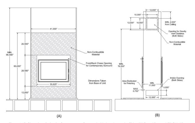
Figure 3-15: Chase Installation for Contemporary Surround with Outtakes at the Side - (A) Front View and (B) Side View
