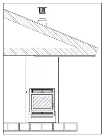
Figure 3-3: Straight Interior Installation
