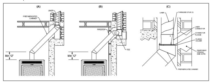
Figure 3-6: (A) Connection into a masonry chimney through an elbow/liner; (B) connection into a masonry chimney through a tee/liner; (C) detailed drawing of masonry chimney connection.
