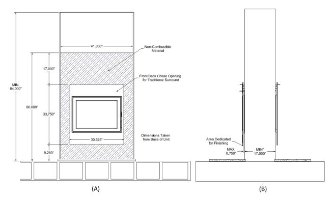
Figure 3-13: Chase Installation for Traditional Surround - (A) Front View and (B) Side View
