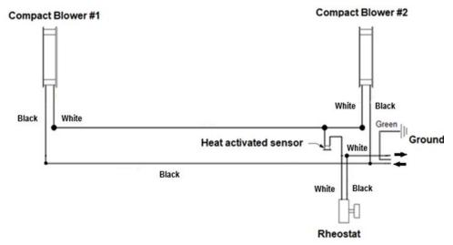
Figure 3-19: Astra Duo Electrical Diagram
