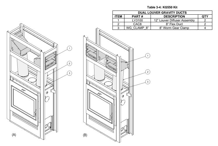
Figure 3-10: Astra Duo 8" Dual Gravity Duct Installation with Outtakes at (A) Side Wall and (B) Front or Back Wall
