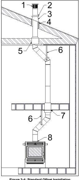
Figure 3-4: Standard Offset Installation
