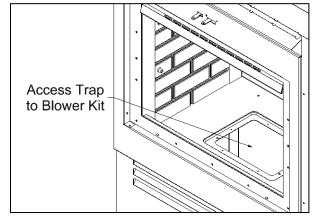
Figure 3-18: Access Trap to Blower Kit
