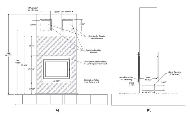
Figure 3-14: Chase Installation for Contemporary Surround with Outtakes at the Front - (A) Front View and (B) Side View
